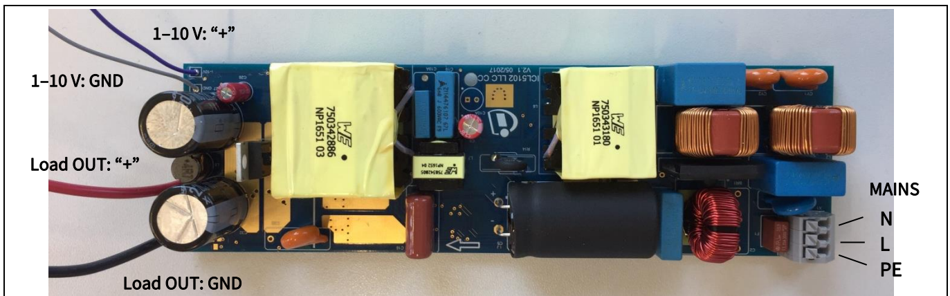
Figure 1 Top view of LED driver connection
